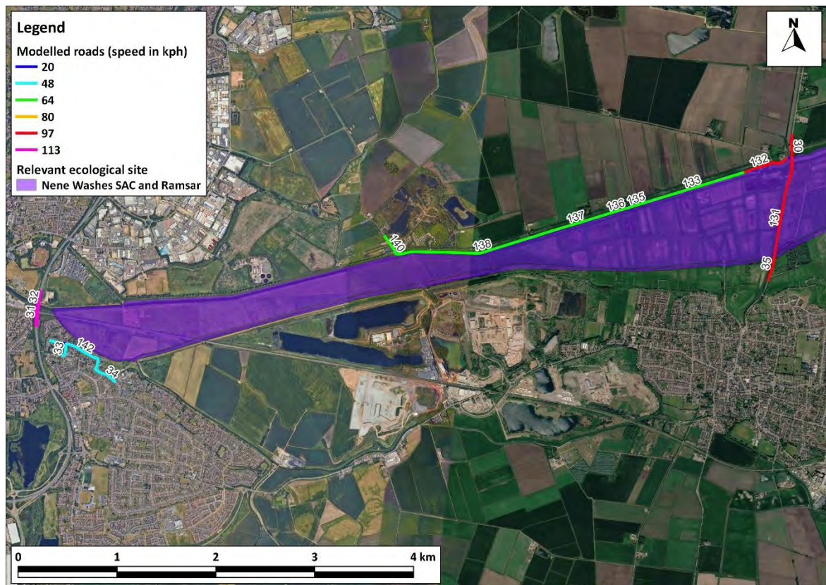
Figure A2-1: Modelled Road Network & Speed – Nene Washes (south)
